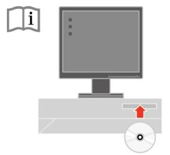
To optimize your monitor image, if using the analog cable, press the Automatic Image Setup key. Automatic image setup requires that the monitor is warmed up for at least 15 minutes. This is not required if you are using the DVI cable.
